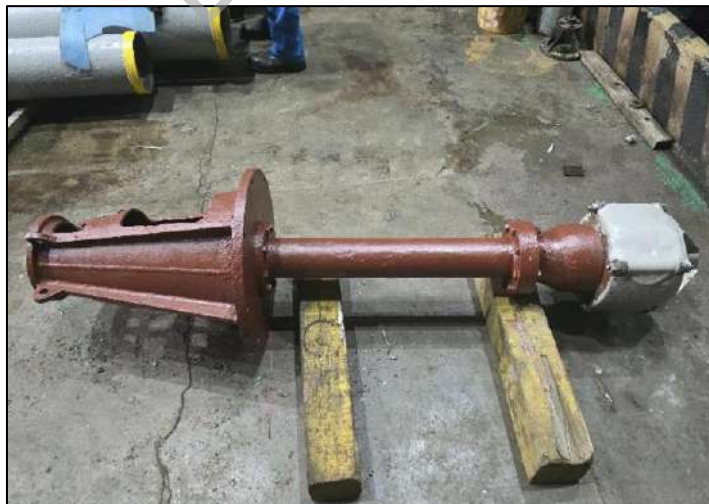
Figure 4: Picture of CWP Recirculation Pump
